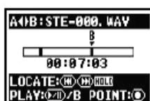
A mark is placed at point A, then mark B appears and moves until set
